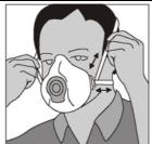
**4.** Ensure respirator fits secure and comfortable. To fasten respirator pull strap at either side of the buckle.
